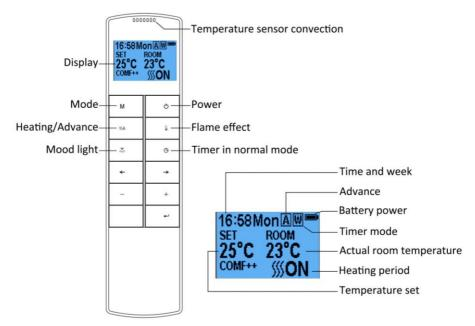
NOTE: This is a thermostatic remote control. The remote should be in the same room as fireplace and placed on a flat surface. It must be placed away from the fire so the hot air will not blow on it and affect thermostatic reading.
